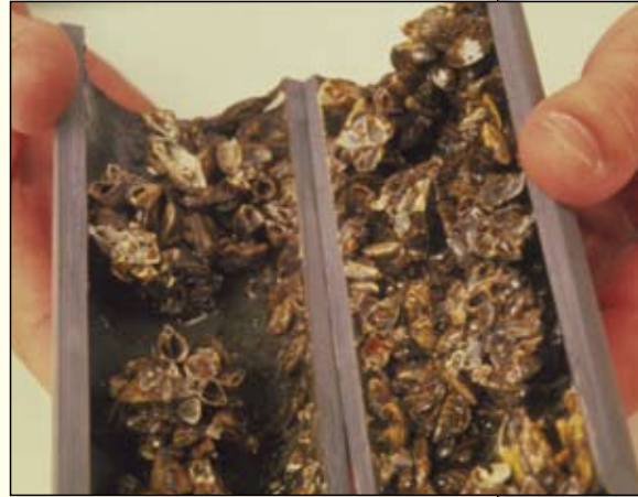
Zebra mussels (Dreissena polymorpha) can clog the insides of pipes.
